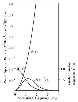
Figure 11-6 Squared transfer function of a Gaussian filter.
