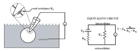
**Figure 1-16** Intracellular electrode measurement. This intracellular electrode is measuring the resting potential of a cell whose membrane contains only open K+ channels. As the seal resistance  $R_s$  increases, the measurement approaches the value of  $E_K$ .
