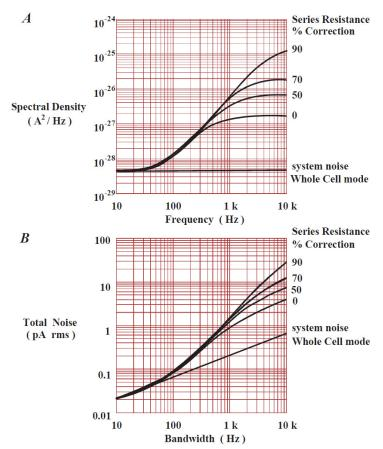
**Figure 11-4** Noise in whole-cell voltage clamping.
