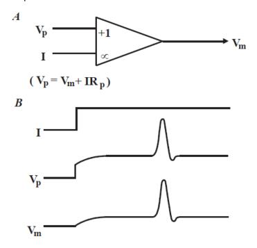
Figure 3-3 The "Bridge Balance" technique.
