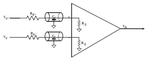
**Figure 7-1** Electrode resistance and cabling can degrade a signal.
