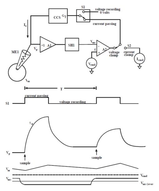
Figure 3-12 Block diagram and timing waveforms.
