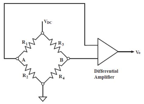
Figure 7-3 Wheatstone Bridge circuit with amplifier.
