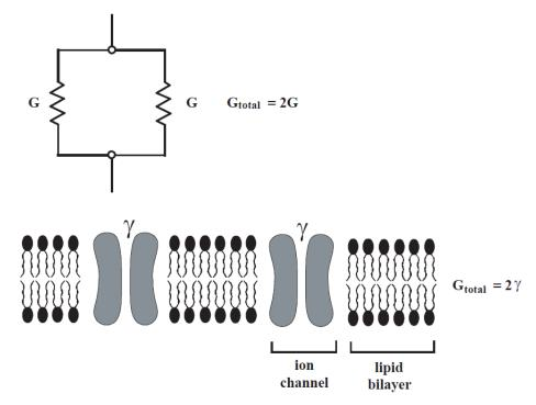
**Figure 1-3** Summation of conductance. Conductances in parallel summate together, whether they are resistors or channels.
