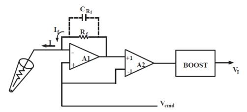
Figure 3-21 Resistive headstage.
