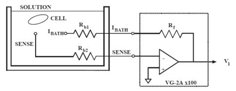
**Figure 3-9** Two-electrode virtual-ground circuit.
