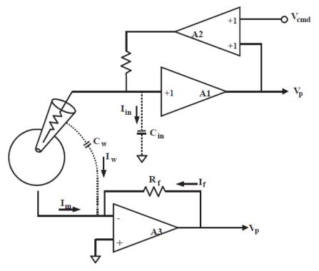
**Figure 3-6** Virtual-ground current measurement.
