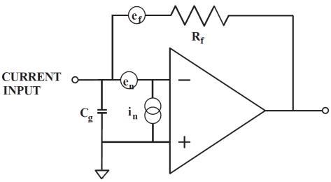
Figure 11-3 Noise model of a simplifier current-to-voltage converter.
