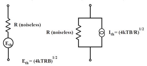
**Figure 11-1** Noise equivalent circuits of a resistor.
