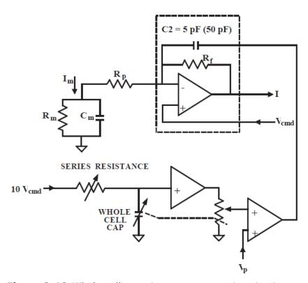
Figure 3-19 Whole-cell capacitance compensation circuit.
