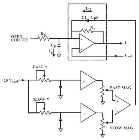
Figure 3-18 Pipette capacitance compensation circuit
