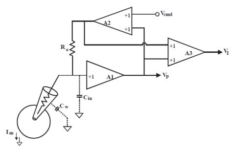
**Figure 3-5** Series current measurement.
