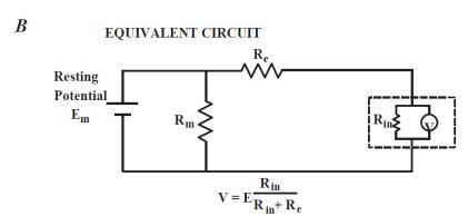
**Figure 1-8** Representative voltmeter with infinite resistance. Instruments used to measure potentials must have a very high input resistance R<sub>in</sub>.
