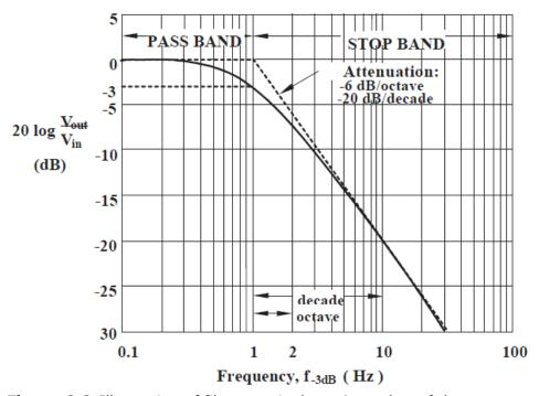
**Figure 6-2** Illustration of filter terminology. A number of the terms used to describe a filter are illustrated in the context of a single-pole, low-pass filter.
