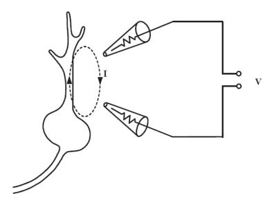
**Figure 1-6** IR drop. In extracellular recording, current I that flows between points of a cell is measured as the potential difference ("IR drop") across the resistance R of the fluid between the two electrodes.
