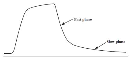
**Figure 3-13** Biphasic voltage response of a high-resistance micropipette.
