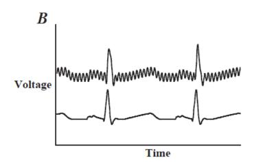
Figure 6-5 Use of a notch filter: inappropriately and appropriately.
