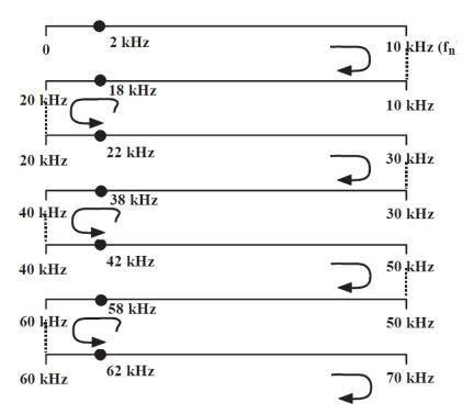
**Figure 11-5** Folding of the frequency axis.
