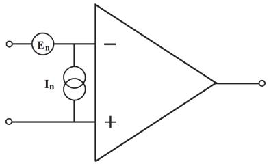
**Figure 11-2** Operational amplifier noise model.
