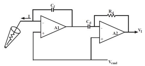
Figure 3-22 Capacitive feedback headstage.
