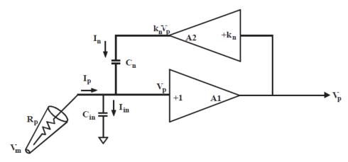
Figure 3-8 Capacitance neutralization circuit.
