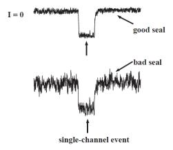
**Figure 1-17** Good and bad seals. In a patch recording, currents through the seal also flow through the measuring circuit, increasing the noise on the measured current.
