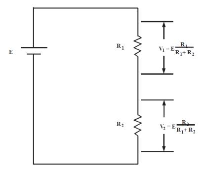
Figure 1-7 A voltage divider.
