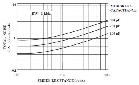
**Figure 3-24** Typical current noise in bilayer experiments.
