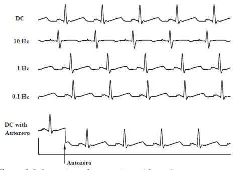
**Figure 6-8** Comparison of autozeroing to AC-coupling.
