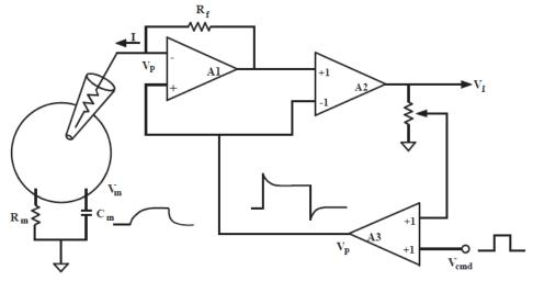
Figure 3-15 Series resistance correction.
