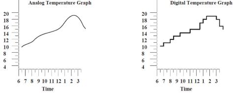
**Figure 9-1** Analog-to-digital conversion.
