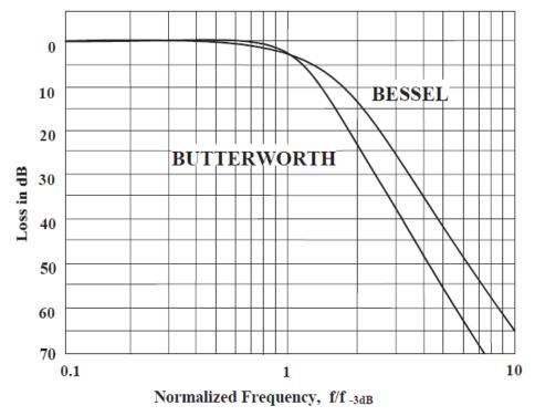
**Figure 6-1** Frequency response of 4th-order Bessel and Butterworth filters. The spectra have been normalized so that the signal magnitude in the pass band is 0 dB. The -3 dB frequency has been normalized to unity.
